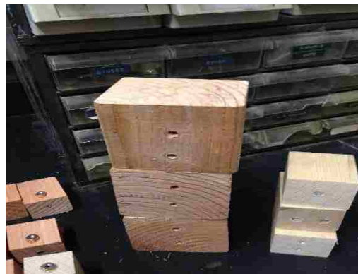
Figure 3-6: Wooden Block Attaches to Side of Pile for Hammer Strike
