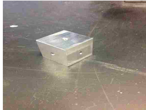
Figure 3-4: Aluminum Block Attaches to Side of Pile for Hammer Strike
