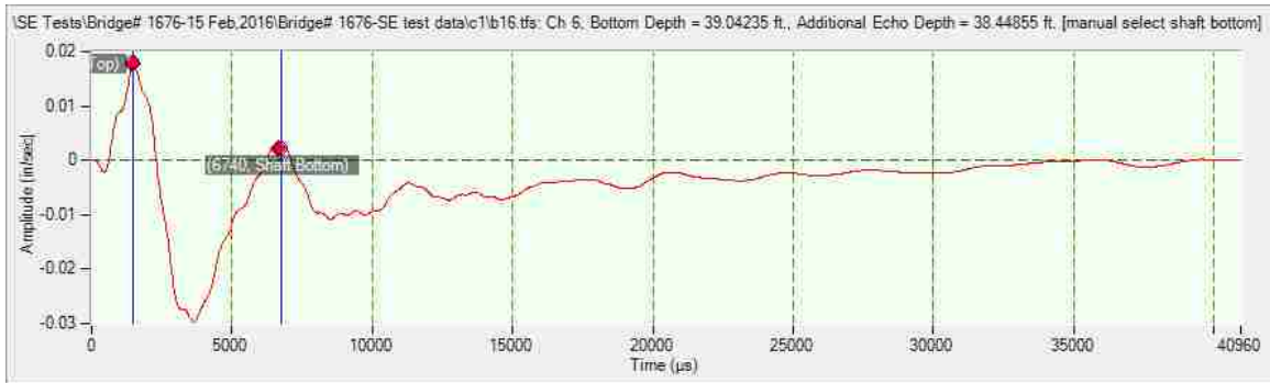
Figure 5-15: Velocity Trace of SE Test No. b16 Using Soft Tip- B Upward
